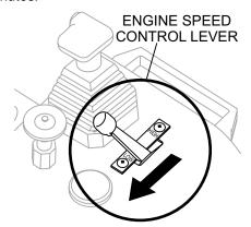
Figure 18. Engine Speed Control Lever Idle (Low Speed)
